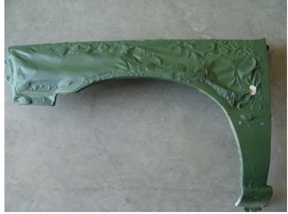
Photograph 2 – Primer and topcoat over previously finished fender, infrared force-dried at 350 0 F for 1 minute
