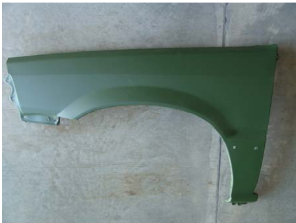
Photograph 3 – Primer and topcoat over previously finished fender, infrared force-dried at 220 0 F for 30 minutes
