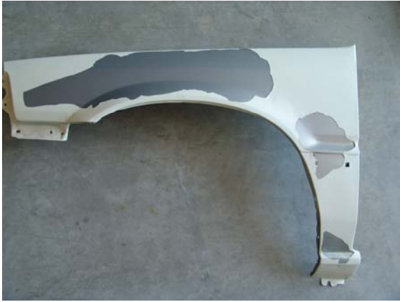
Photograph 1 – Primer over previously finished fender, infrared force-dried at 325 0 F for 1 minute
